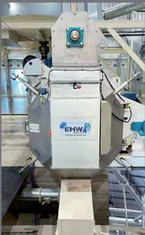
EHW Italia has presses of different sizes and capacities: the diameter of our dies starts from 420 mm up to 1,200 mm, the main motors range from 75 to 630 kW for a production capacities from 0,8 to 10 tons/h.
