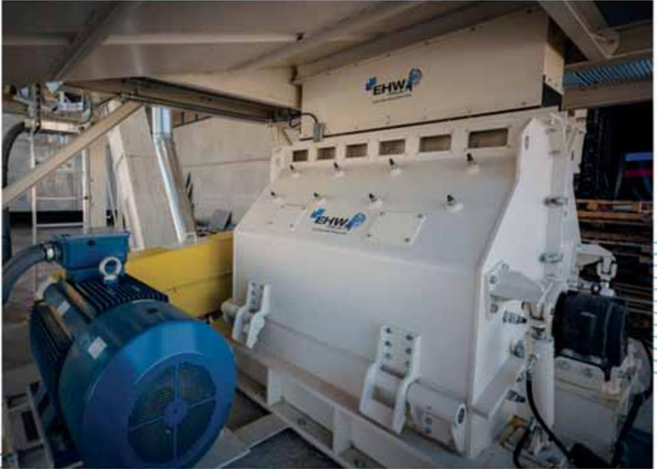
Our hammer mills, equipped with robust frames, are ideal for reducing and grinding raw material, both wet and dry, to an ideal grain size.
