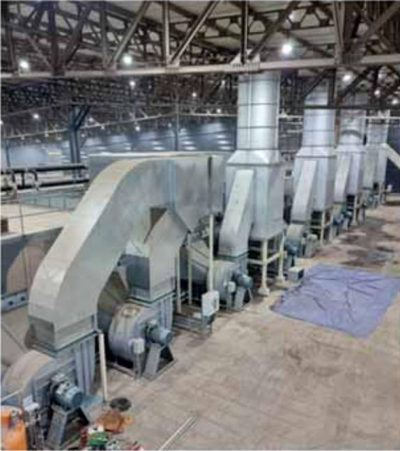
They consist of loading bunkers with screw feeders, which ensure homogeneous product distribution on the belt, a drying tunnel complete with dust extraction and belt centring systems.
