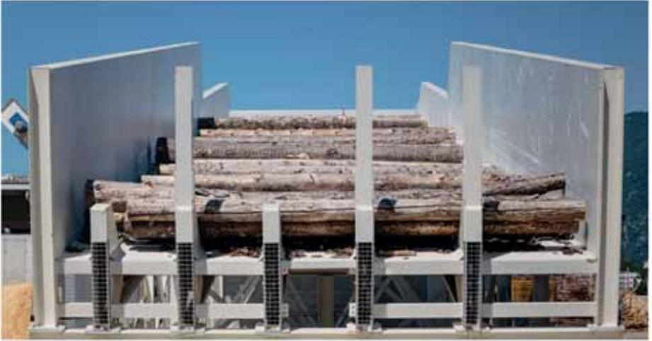
EHW's log debarker is conceived to be able to work with logs of various lengths and is specially designed for debarking curved and knot-marked logs.
