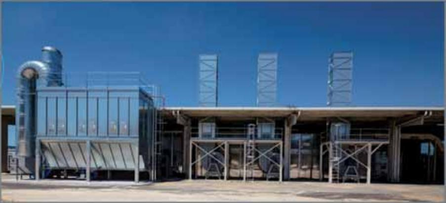
The belt drying system, with no direct contact with hot fumes, eliminates the risk of fire during the work cycle.
